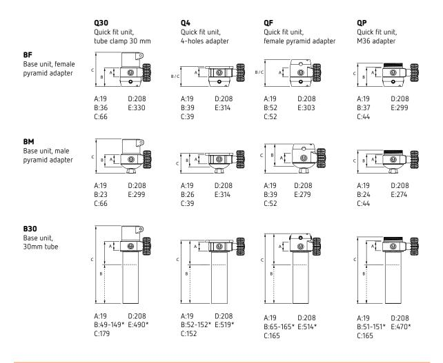
**A** Functional height in mm **B** Effective height in mm **C** Total height in mm **D** Effective weight in g **E** Total weight in g \*B30: Adaptable effective height and weight as tube can be cut off with up to 100 mm.
