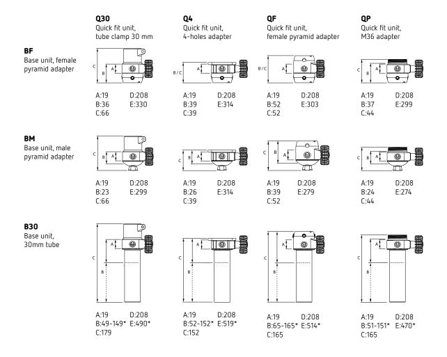
**A** Functional height in mm **B** Effective height in mm **C** Total height in mm **D** Effective weight in g **E** Total weight in g \*830: Adaptable effective height and weight as tube can be cut off with up to 100 mm.
