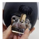
When everything is installed, use Loctite to lock the prong adapter. This must be done before the patient walks on the prosthesis.
